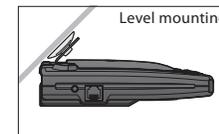
When installed and adjusted properly, the back top edge of PASSPORT should rest solidly against your windshield.
